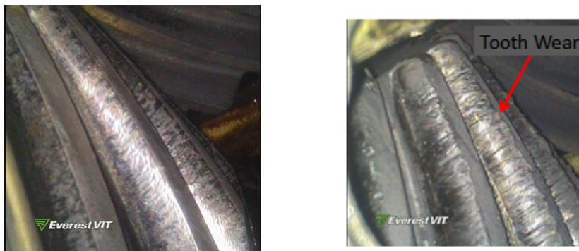
Figure 6.3: Earlier stage of testing (left)and after failure (right)
